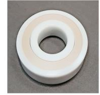
for extremely low temperatures. SMB ceramic bearings are usually dry but we can lubricate them to order if required. Ceramic bearings with cages are stocked as open or with PEEK seals (2PKS). We can supply them with PTFE seals for extreme low temperature applications. Full complement bearings are only available open.
